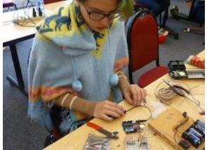
Attaching a microprocessor to the plotter and changing the variables on the Arduino sketch allowed different designs to be drawn automatically.
